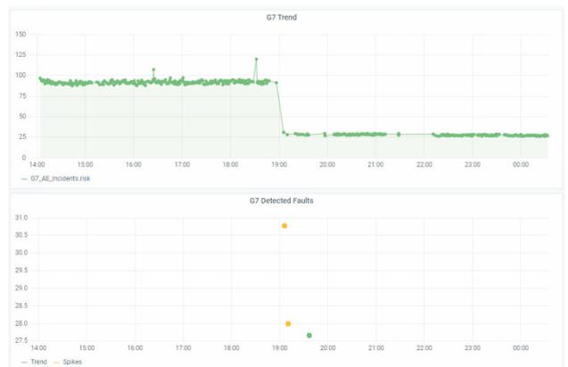
Fig. (7). Fault Detection on Acoustic Emissions - Different Modules Deviation. The change of the module is applied in the middle of the figure. The graph in the bottom depicts the points where anomalies are detected.
