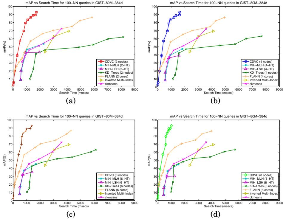
Fig. 5. Comparison of CVDC on the **GIST-80M-348d** evaluation dataset against MIH-LSH, MIH-MLH, distributed KD-Trees over the cloud (KD-Trees) and FLANN for (a) 2, (b) 4, (c) 6 and (d) 8 nodes / Hash Tables (HT) / CPU-cores. The performances of Inverted Multi-Index and ckmeans are preserved by varying the number of nodes, since both methods do not work in parallel.
