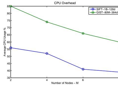
Fig. 8. (a) CPU Overhead/Usage (%) of an *Image Sorter* node in GIST-80M-384d and SIFT-1B-128d, by varying the number of the  $M$  nodes over the cloud infrastructure.
