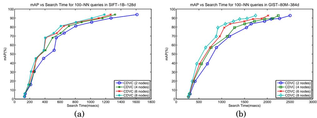
Fig. 9. Performance of CDVC on the cloud infrastructure for (a) SIFT-1B-128d and (b) GIST-80M-384d.
