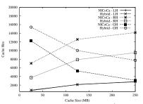
Figure 3: Impact of cache size on hits (large multimedia files and uniform access) in a dense WMSN (d = 7).
